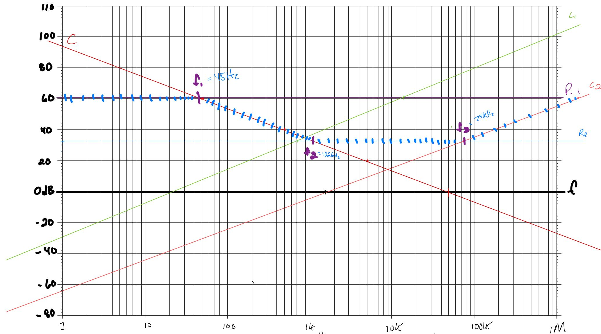
$$C \text{ crosses axis} @ \frac{1}{2\pi \cdot 3.3 \times 10^6} = 48.285 \text{ Hz} \\ R_2 \text{ crosses } C @ \frac{1}{2\pi R_2} = 1026 \text{ Hz} = f_1$$
