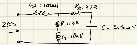
$$L_2 + (R_2 \parallel C) \parallel (R_1 \parallel L_1)$$
